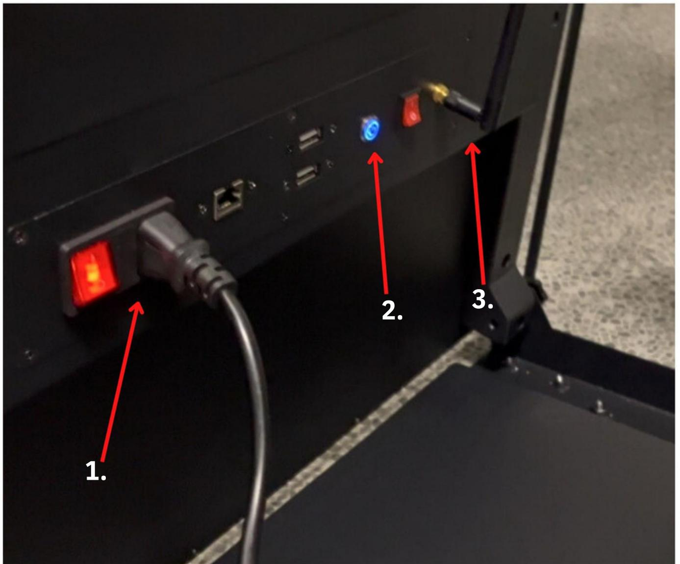
**1. We connect the source cable from the socket to the photo booth and press the switch.**
